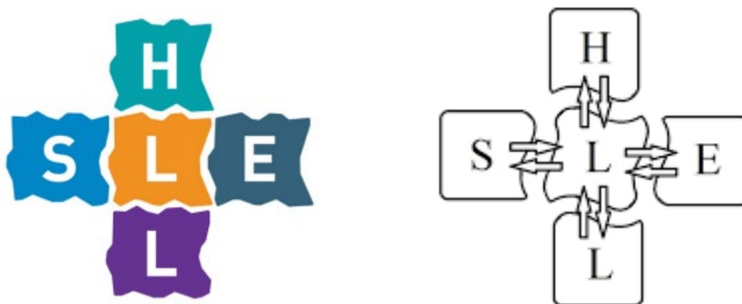
Figure 12 – Scheme of the SHEL conceptual model proposed by ICAO for human factors research (Edwards & Hawkins)
