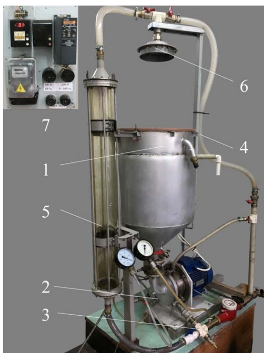
Figure 1 - Aeration and oxidation installation of the rotor type:
