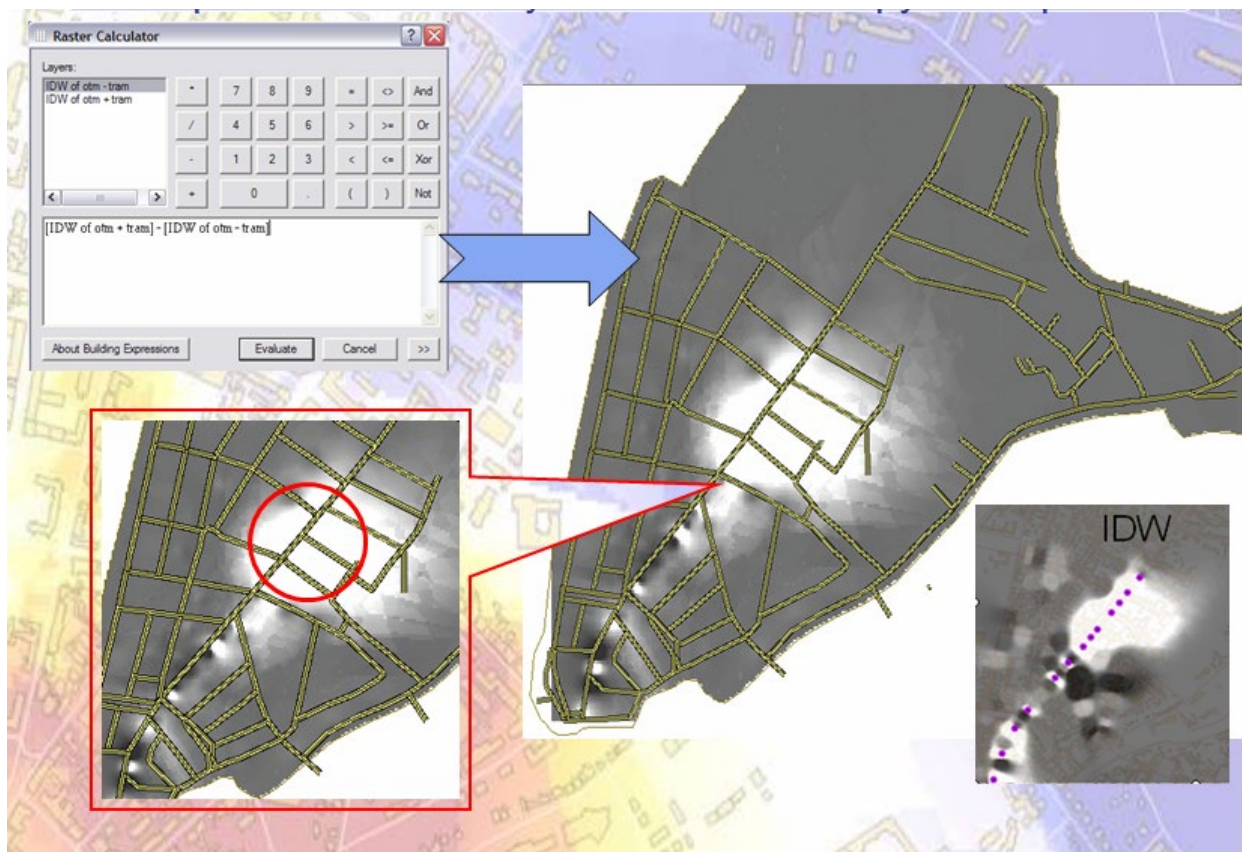
Figure 8 – Creation of a model of noise pollution of the "Tram" layer using GIS tools
