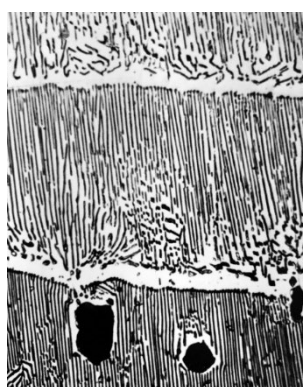
Figure 6 – Structural changes at the growth front of austenite-carbide colonies during thermal cycling; electrolytic etching; \times 630
