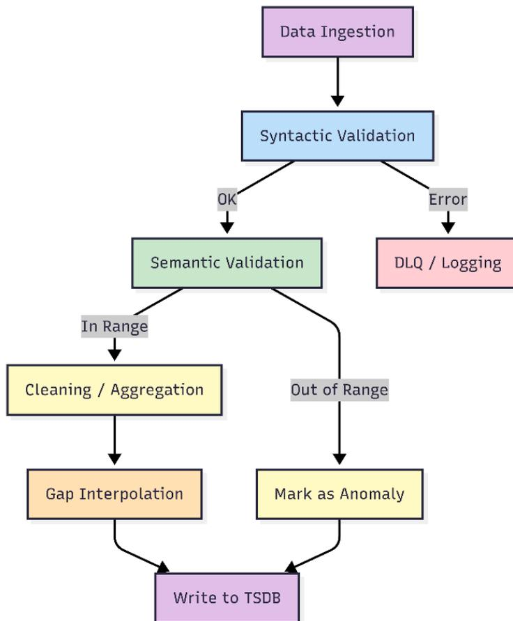
Figure 6.1 – Sequence of Data Validation and Cleaning Steps
