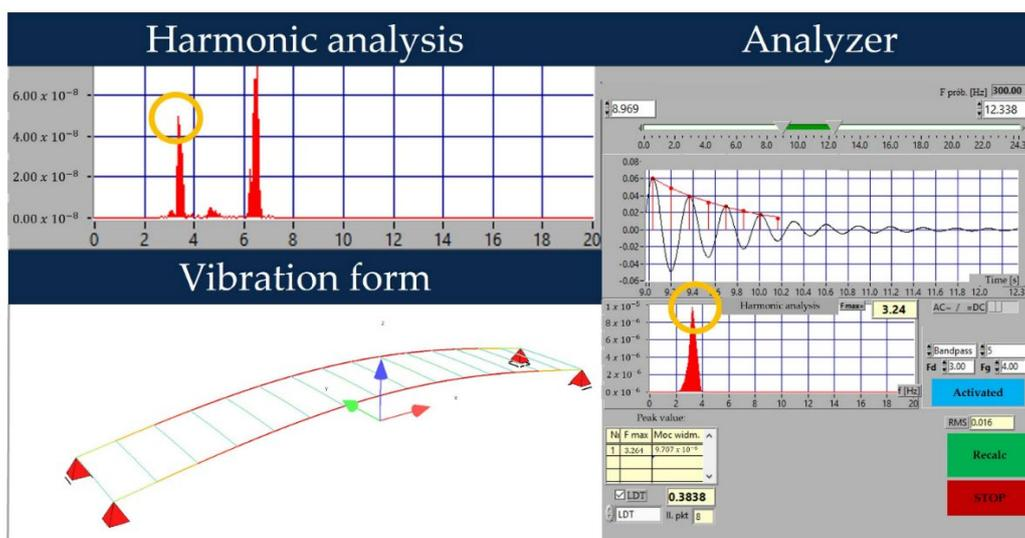
**Figure 3.2 - Identification of natural frequencies and corresponding damping.**
