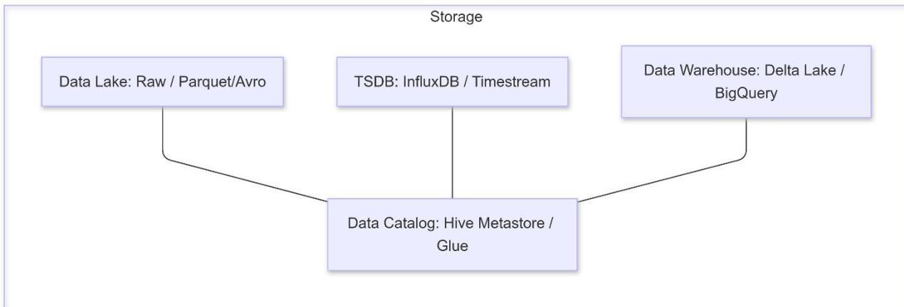
**Figure 6.2 – Interaction Between Data Storage Layers and the Metadata Catalog**
