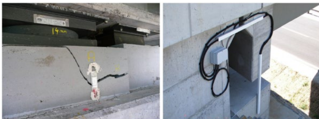
Figure 5.1 – Examples of Fiber Bragg Grating (FBG) Sensor Applications
